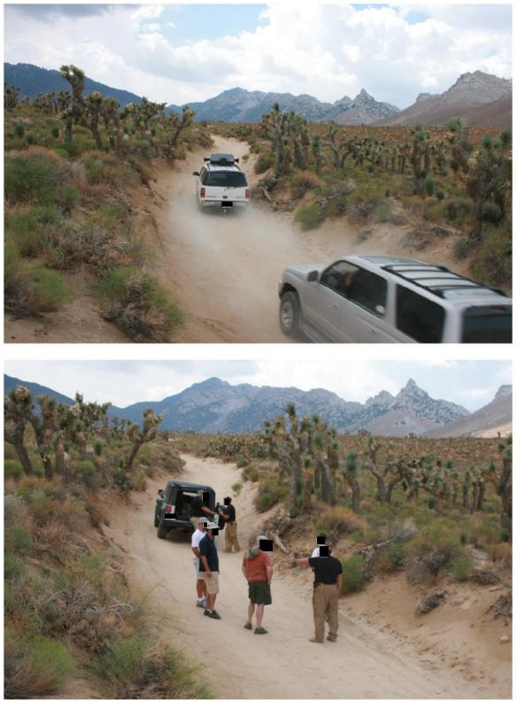
Terrain Chosen: Worst of all conditions; Double hair-pin turns, vehicle forced to present broadside multiple times throughout turns; vehicle front end angled up approximately 15° with respect to the threat device; banks, washes, and
